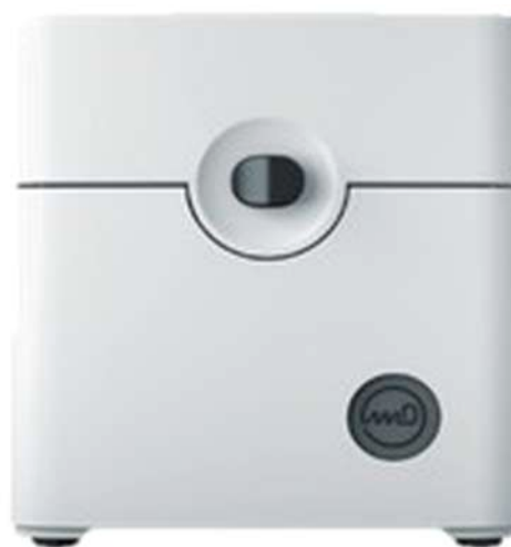
Fig. 2. Instrument in use for on chip qPCR amplification step. The dimensions are 16 \times 18 \times 16 cm (length \times height \times width).
